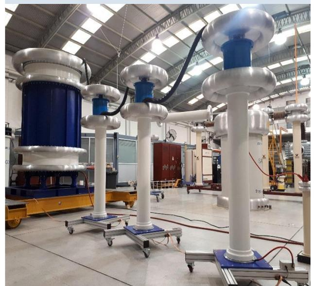
LABORATORIO INDUCOR-UTNLAT - NUEVO REACTOR RESONANTE 4MVA-220KV S/IEC60840 / IEC62067
