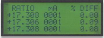
The ATRT-03 can also calculate the turns-ratio percentage error if the transformer's nameplate voltages are provided. The baseline turns-ratio is calculated using the nameplate voltages, and the test results are compared to the baseline turns-ratio. The percentage error is then calculated from the difference between the baseline and test turns-ratios.
