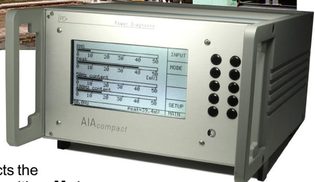
UHF measurements on embedded or external sensors are possible with the use of the RPA6C, a logarithmic preamplifier, which covers 300MHz-2GHz. As with the other preamplifiers, the AIAcompact automatically detects the RPA6C and changes into the logarithmic display for the UHF detection. Generally, the instrument offers three main display modes, which are selected using dedicated control buttons: Scope, Meter, and Time.
