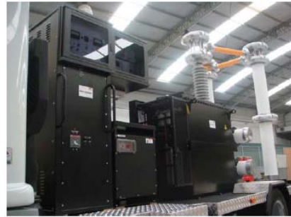
220 kv VLF-200 HVCD mobile unit, with Tangent Delta/Partial Discharge test capacity (INDUCOR INGENIERIA S.A.)
